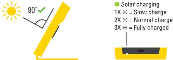
Position the WakaWaka Light facing the sun at an angle of 90 degrees for maximum charge speed. The WakaWaka Light charges in 5-8 hours in the sun.
